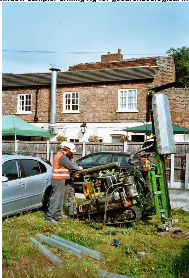
Figure 9 Use of a window sampler drilling rig for geoarchaeological investigation
